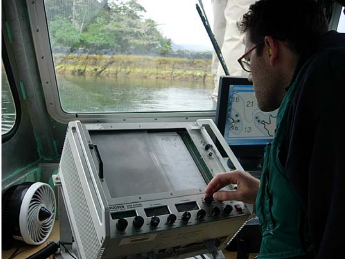
ENS Jamie Wasser, monitoring the Echosounder onboard RA1 during investigative surveys.
