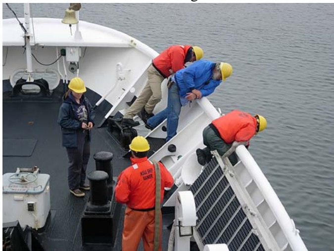
RAINIER deck crew looking over the side of the ship to watch the anchor as it is being lifted out of the water. Communication from the deck to the bridge on the location of the anchor relative to the ship's position is important to prevent damage of the ship's hull.
