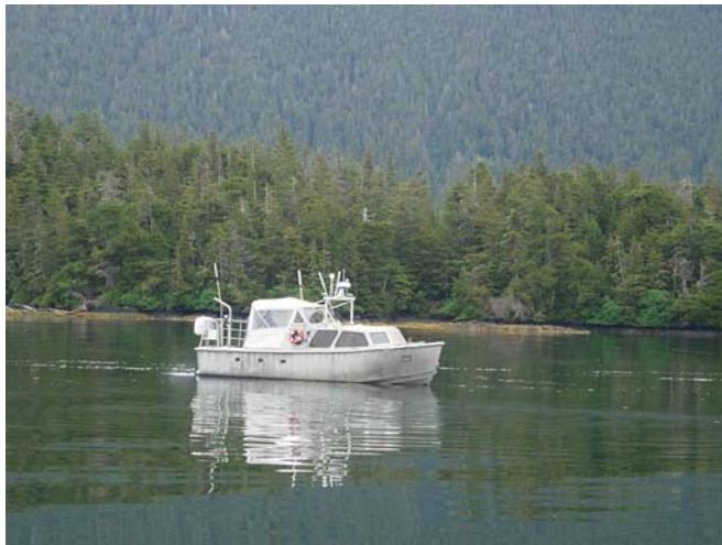
Survey launch RA5 working in Kanga Bay in Southeast Alaska. The cruising speed of RA5 is up to 25 knots, but while on the survey line logging data, the boat can go no more than 8 kts.
