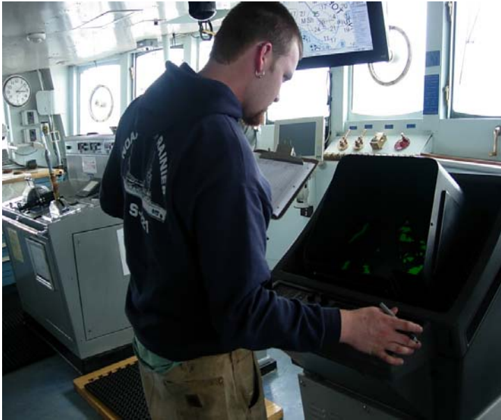
On the bridge, General Vessel Assistant, Kelson Baird is logging the ships position from four points on the radar screen. The position of the points is recorded every half hour to monitor the effectiveness of the anchor.
