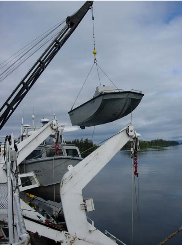
The 3,000lb skiff is being lifted up and over one of the survey boats off of NOAA ship RAINIER. The skiff will serve as a rescue boat in case of an emergency while the survey boats are collecting data near the bay.
