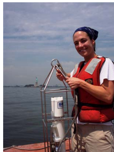
TAS Candice Autry prepares to use the CTD instrument which collects water information related to conductivity, temperature, and depth.
