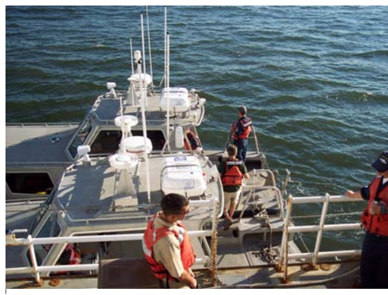
Crewmembers of the THOMAS JEFFERSON prepare the launches to set forth and collect data using side-scan sonar and multi-beam sonar.
