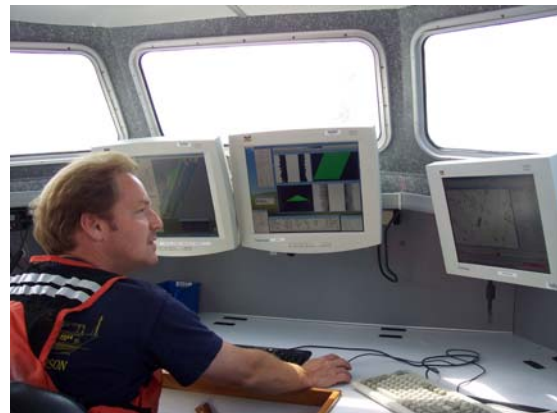
Surveyor Doug Wood observes four computer screens where data is being collected. The green triangle seen on the computer screen is showing multi-beam sonar information being collected. Multi-beam sonar provides the depth information for any obstruction.
