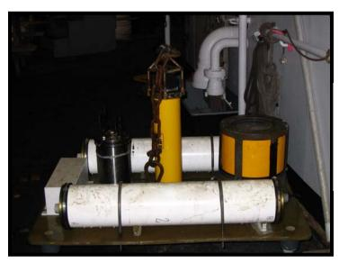
The BPR immediately after recovery, without its anchor that remains on the bottom of the ocean.
