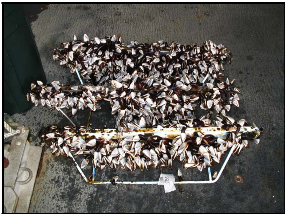
Stratus 6 instruments one year after deployment covered in barnacles. What would two years of deployment look like?
