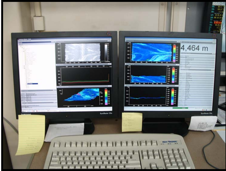
Before scientists deploy a buoy they must measure how deep the ocean is. This is the actual bathymetric (bottom measure) read out of the target site for Stratus 7.
