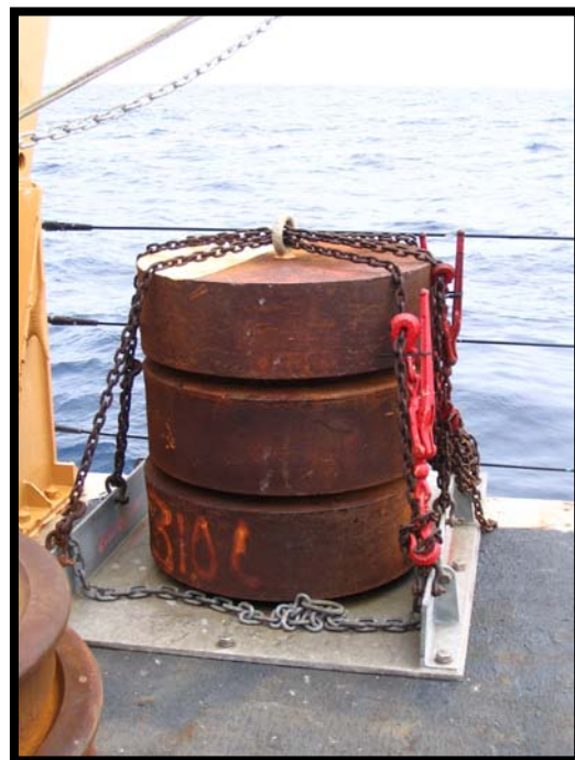
The anchor for the buoy
