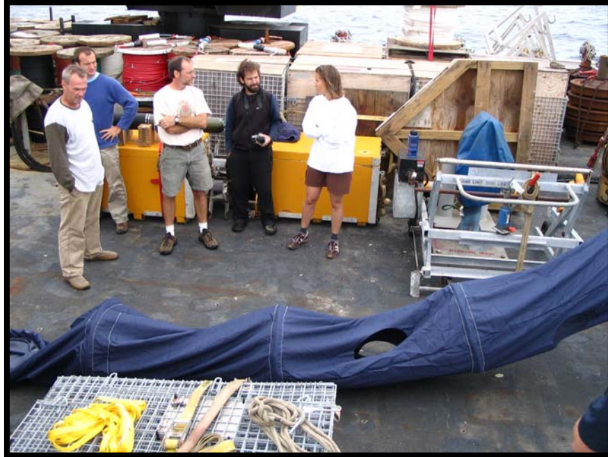
This is the drogue chute that is deployed in the water beneath the drifter to stabilize its deployment with the ocean currents.
