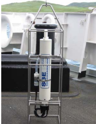
A CTD, which gets lowered into the water prior to beginning surveys to get a reading on the speed of sound through the water.
