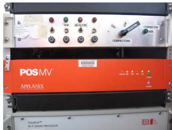
The POS MV aboard one of the NOAA ship RAINIER survey boats.
