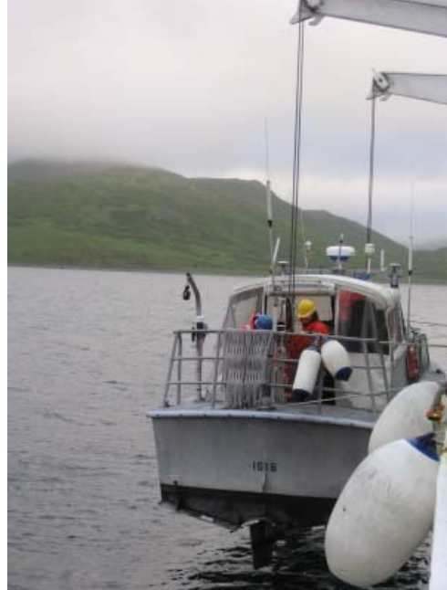
Lowering a survey launch off of NOAA ship RAINIER
