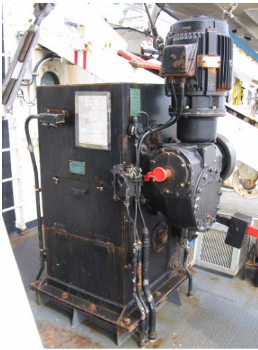
Davit winch, which helps to move the survey launches.
