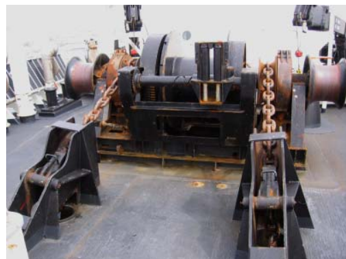
The anchor windless on NOAA ship RAINIER. Each chain is about 1080 feet long. The anchor itself weighs about 3500 pounds.
