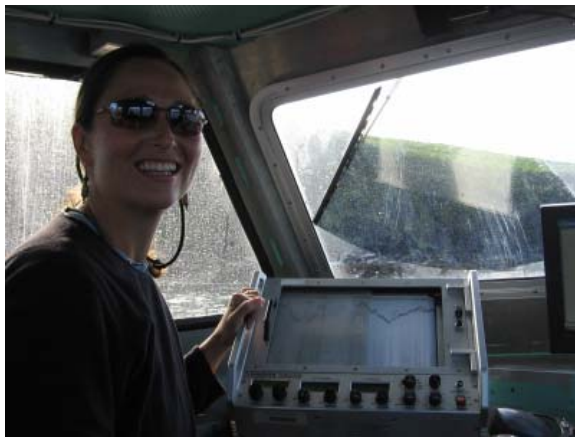
TAS Kim Wolke operating the echosounder on a hydrographic survey of the Shumagin Islands in Alaska
