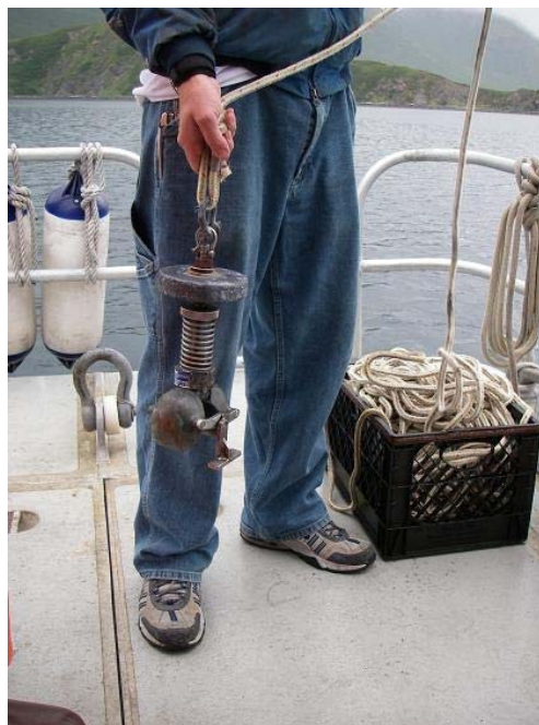
A lead weight is fastened to the end of the bottom sampler.
