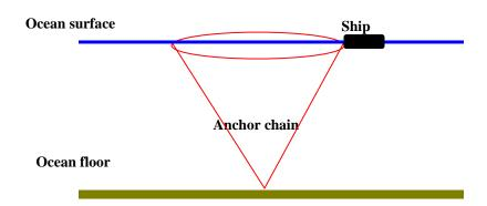
This diagram show the coneshaped pattern that the chain will move in as the ship swings around at anchor.
