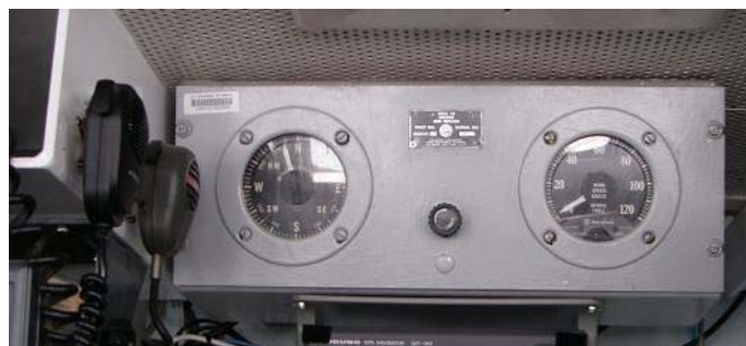
An anemometer measures wind speed.
