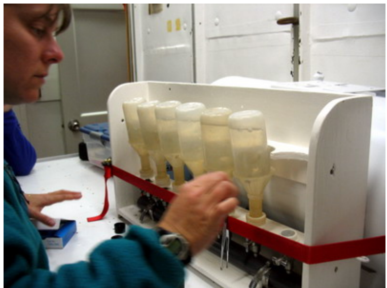
Water samples being filtered through a vacuum system to extract chlorophyll.
