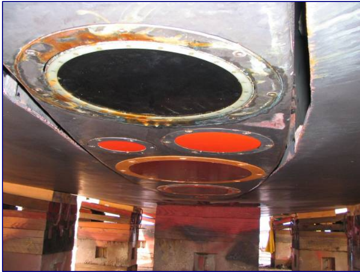
Picture of the transducers in the centerboard, which is lowered when the ship is at sea. Lowering the transducer away from the hull reduces the noise interference of bubbles running along the hull while underway.
