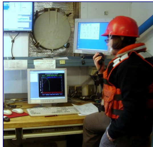
Above: Survey Technician Tayler Wilkins monitors the CTD data transmission while communicating with the crane operator as the rosette is lowered through the water column. The computer automatically produces a profile of temperature and salinity with depth.
