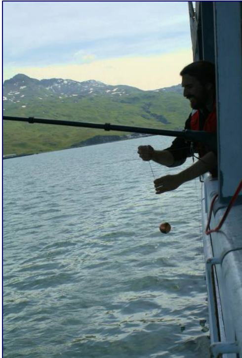
Chief Scientist, Patrick Ressler, attaches calibration spheres to the line that will be lowered beneath the ship.
