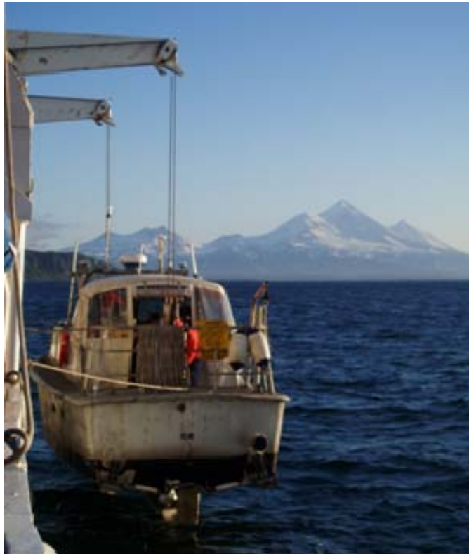
Lowering a launch using a gravity davit system
