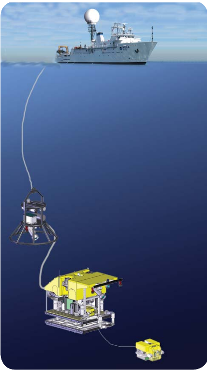
The bell-shaped camera sled, the science-class ROV and the small xBot can operate as deep as 6000 meters. NOAA illustration with vehicle drawings by ROV builder Phoenix International.
