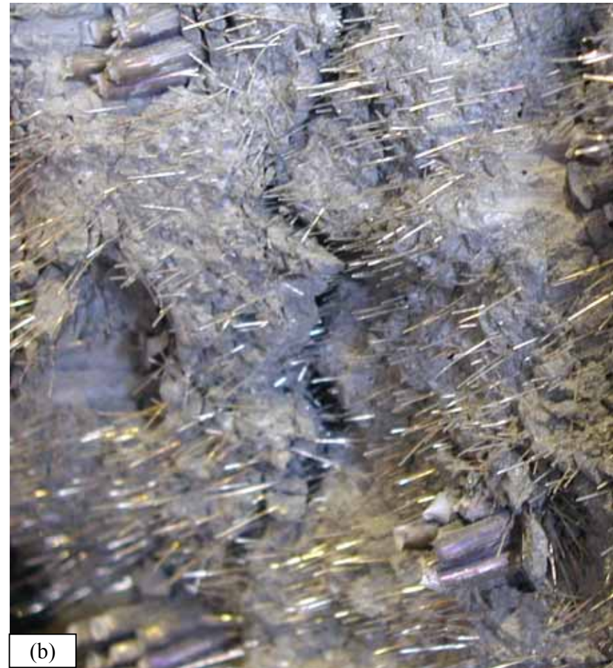
Figure 19. Photo. Failure surface of Girder 80F including (a) overall west failure surface and (b) closeup of west failure surface showing pulled-out fibers and necked strands.
