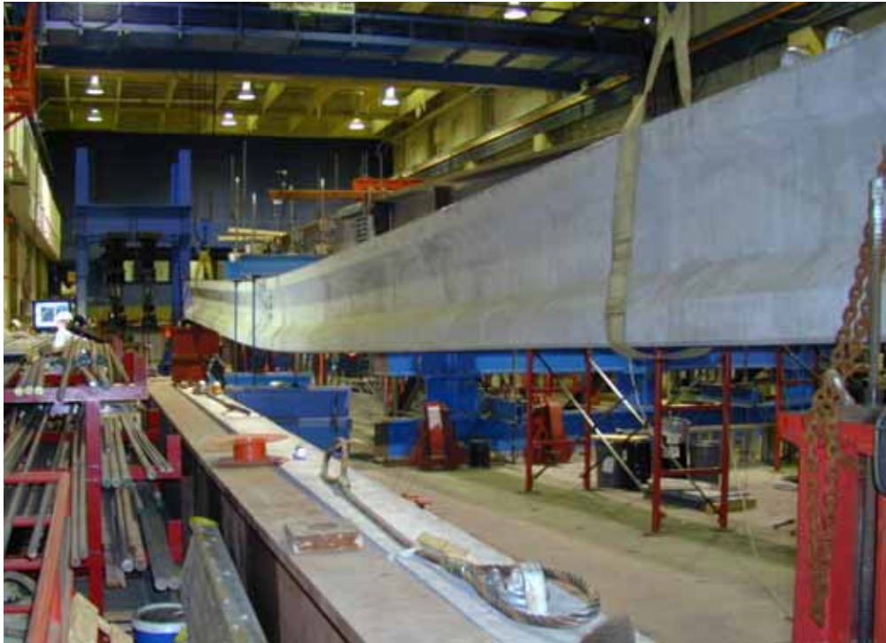
Figure 17. Photo. Girder 80F after approximately 430 mm (17 inches) of deflection.
