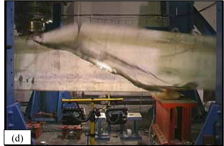
Figure 38. Photo. Failure of Girder 24S (a) 1/15 second before failure, (b) 1/30 second before failure, (c) at failure, and (d) 1/30 second after failure.
