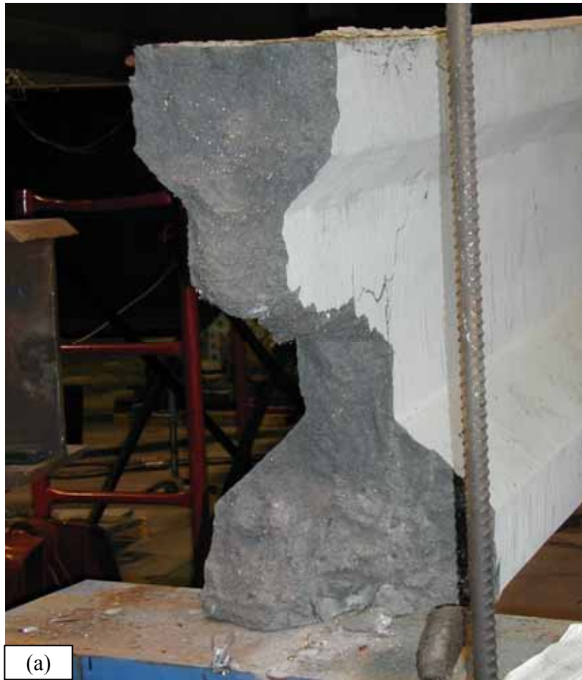
Figure 19. Photo. Failure surface of Girder 80F including (a) overall west failure surface and (b) closeup of west failure surface showing pulled-out fibers and necked strands.
