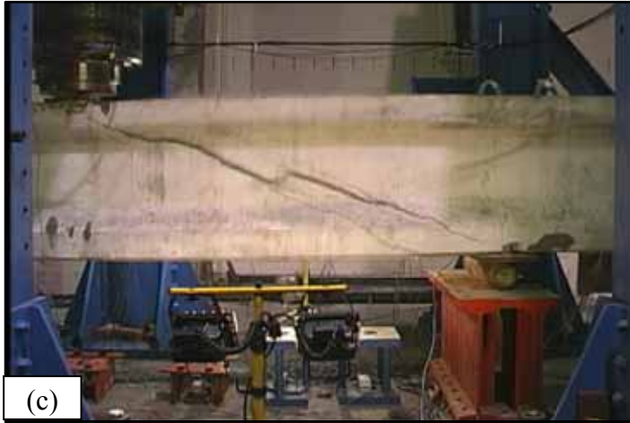
Figure 38. Photo. Failure of Girder 24S (a) 1/15 second before failure, (b) 1/30 second before failure, (c) at failure, and (d) 1/30 second after failure.
