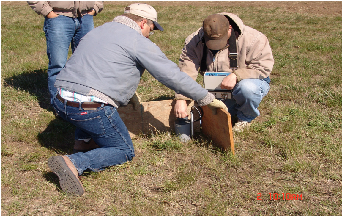
Figure 1. Soil surface CO 2 flux measurement with Environmental Gas Monitor chamber and data logger
