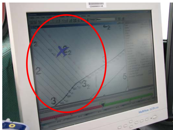
The lines circled in red are the track that the boat follows back and forth in order scan the bottom of the sea. It's a lot like mowing a lawn!
