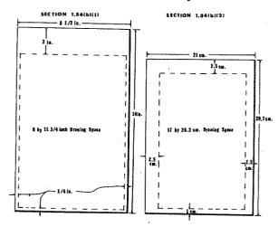
Design patent drawings, 37 CFR 1.152, § 1503.02.
