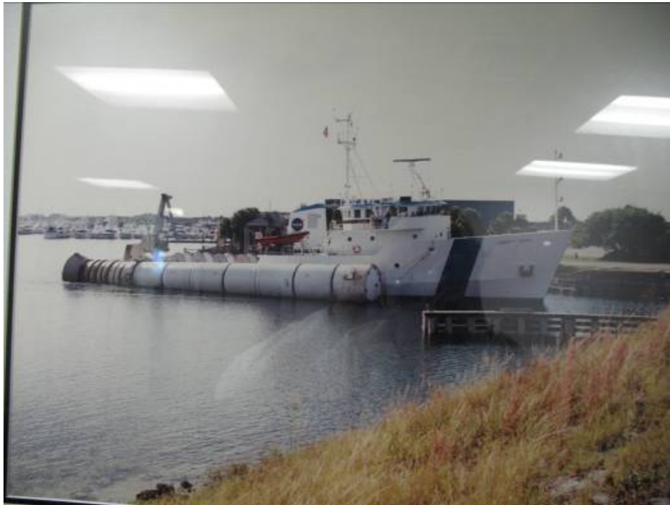
A picture of the LIBERTY STAR with the space shuttle rocket boosters on her starboard side
