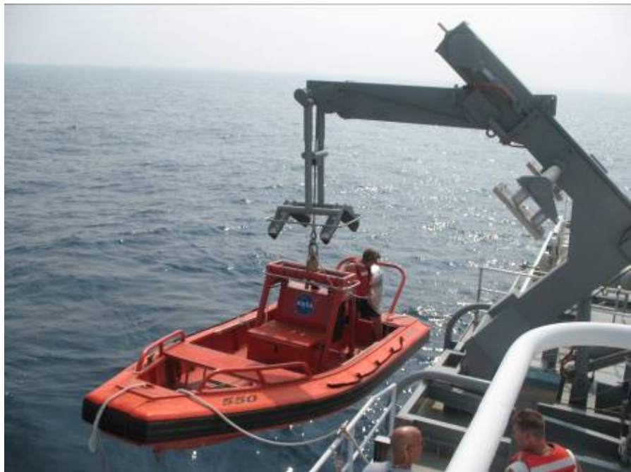
A small boat on the LIBERTY STAR had to be deployed to untwist the ROV cord from the ship's propeller.
