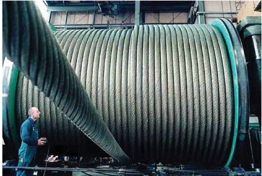
Above: Cable used for moorings.
