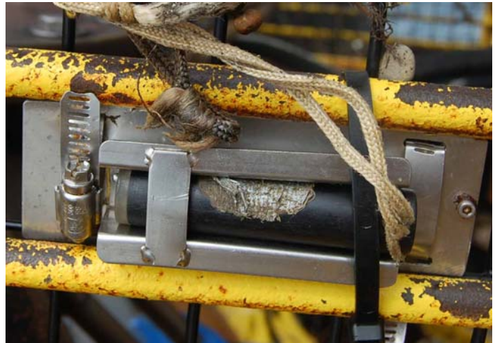
Two small black tubes (~3 inches long), called miniloggers, are attached to the dredge. The miniloggers measure the manifold (inside) and ambient (outside) pressure and temperature during the tow.
