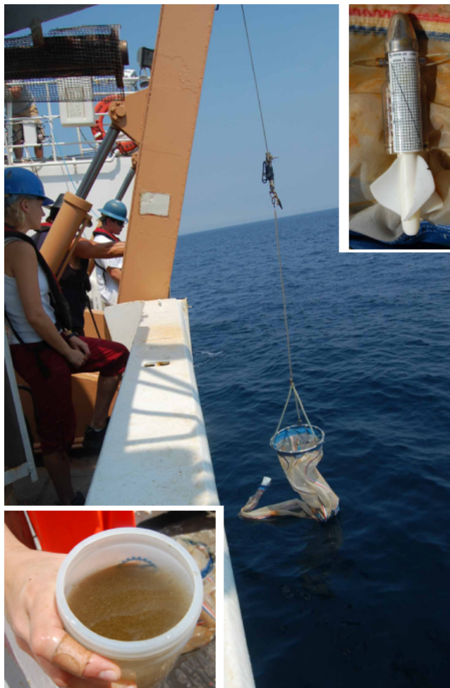
NOAA Scientist Amy Nau hauls the plankton net out of the water using the A-frame. (Upper insert: flow meter; lower insert: plankton in the collection bottle after the tow).
