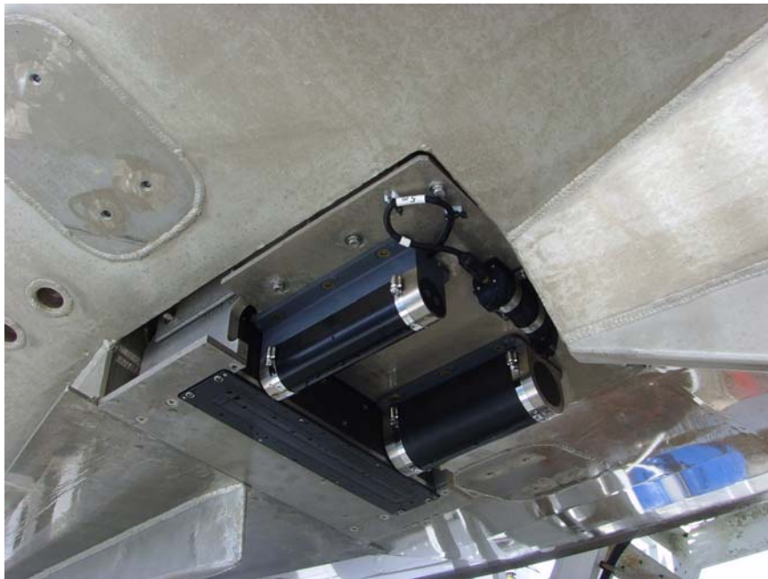
This is the Reson Sea Bat 7125, the type of sonar on the bottom of one of the RAINIER's launches.
