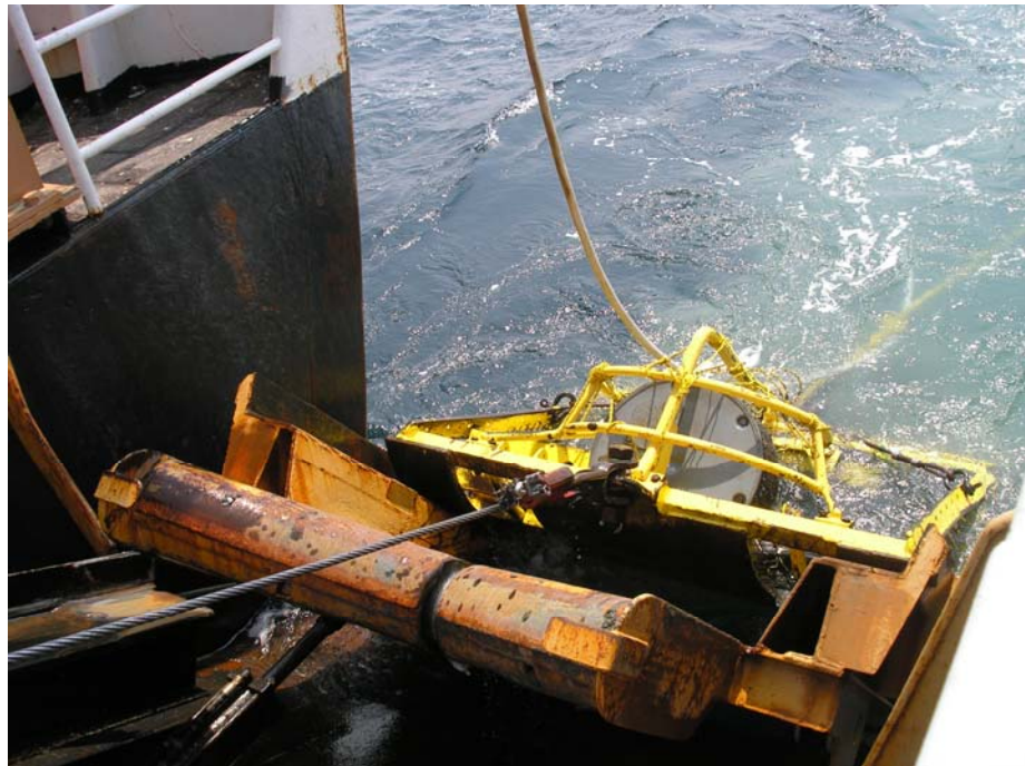
The dredge being brought back up onto the ship after being deployed
