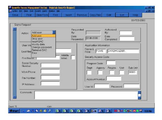
The ACTION is the first field on the request screen. Press the **[Down Arrow]** to the right of the field to see a drop-down list of valid action codes:
