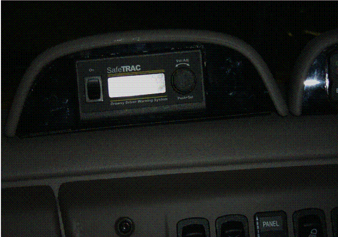
Figure E-5. SafeTRAC™ Pod Mounting Position
