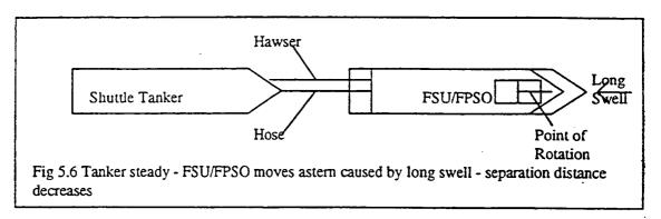
In the figure above the FSU/FPSO begins to move astern. The movement is caused by the combined effects of the long swell on the subsea mooring system and on the hull form of the FSU/FPSO. The tanker remains steady. The astern movement of the FSU/FPSO has reduced the separation distance to 60 metres.
