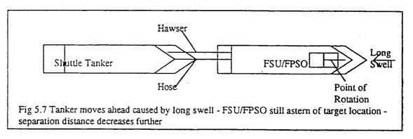
In the figure above the FSU/FPSO remains steady in position offset some 10 metres astern of its target position. In the meantime the swell has acted on the more responsive shuttle tanker which surges ahead some 20 metres, thus reducing the separation distance to 40 metres.
