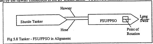
In the figure above there is no relative movement at the DP shuttle tanker - FSU/FPSO interface. The separation distance is steady at 70 metres. There is 10 metres slack in the hawser.
