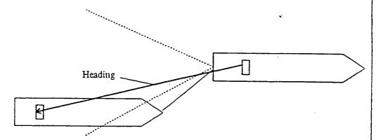
The figure above provides an additional application of the sector excursion limit. In this case the tanker's heading is in alignment with the FSU/FPSO, but the bow of the tanker is outside of the sector limits. This can also result in an alarm condition.
