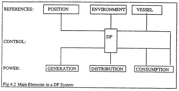
The most important parts of the DP system are those which are common to several major items of equipment and, no matter how much redundancy is provided, some elements of control are inevitably common.
