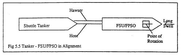
In the figure above there is a long swell but there is no relative movement between the tanker and the FSU/FPSO. Assume that the separation distance is steady at 70 metres. The hawser is slack.
