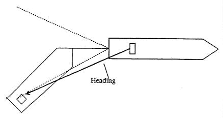
The figure above illustrates the shuttle tanker heading outside the heading alarm limits and the DP system responds by applying appropriate thrust to enable the tanker regain appropriate heading.
