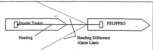
The figure above shows the shuttle tanker and the FSU/FPSO in alignment. The heading information is transmitted from the FSU/FPSO to the shuttle tanker by the UHF link for the DARPS unit. Ideally there should also be a secondary transmittal of the heading information. This can be achieved via the Artemis link.
