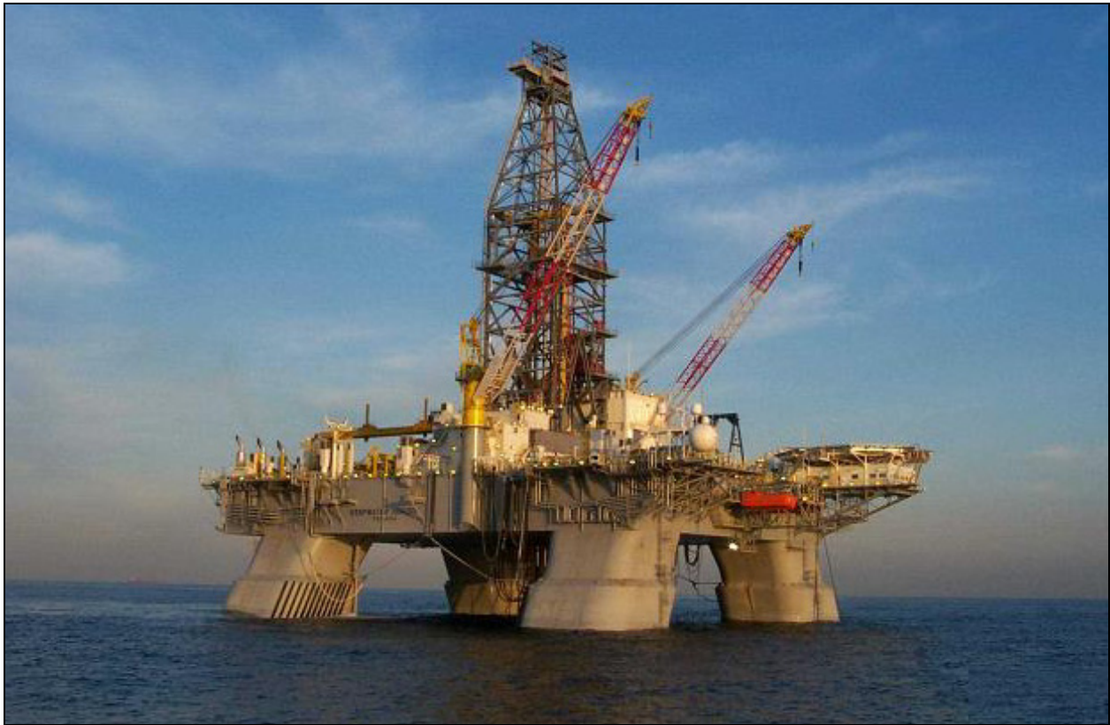
Figure 19. The Deepwater Horizon , a dynamically positioned, semisubmersible drilling unit (photo courtesy of Transocean).
