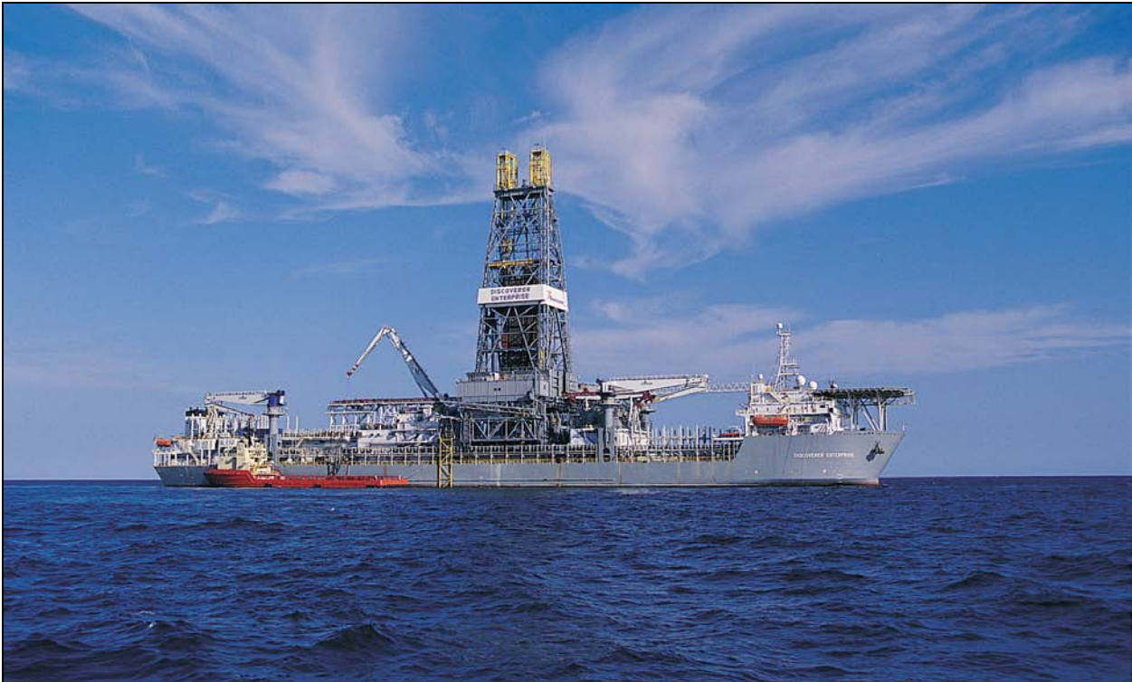
Figure 20. The Discoverer Enterprise , a double-hulled, dynamically positioned drillship (photo courtesy of Transocean).
