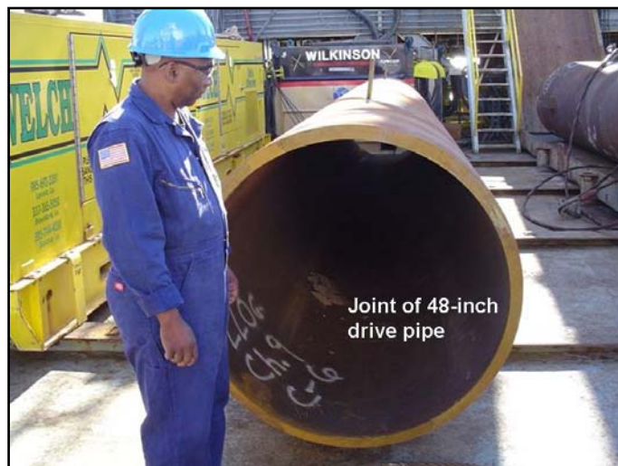
Figure 5: Example, 48-in drive pipe
