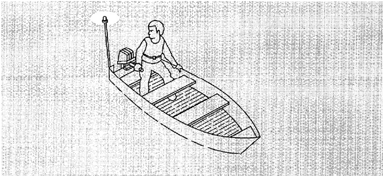
Power-driven vessel of less than 7 meters in length whose maximum speed does not exceed 7 knots.
