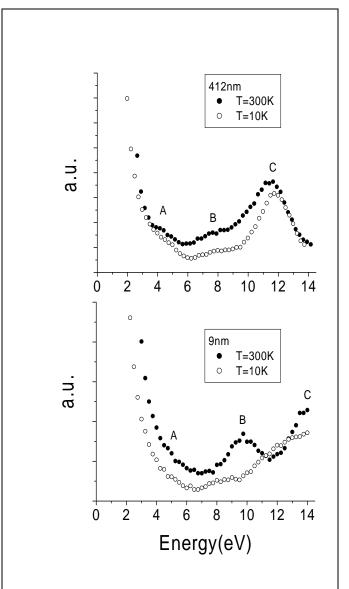
Fig. 1. RIXS measurements of 412nm (top panel) and 9 nm  $La_{0.8}MnO_3$  films (lower panel) showing the strain induced localization of 3d band (labeled B) in the insulating phase of the 9 nm film. (APL **90**, 101915, 2007)
