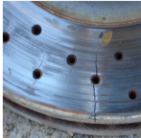
Figure II-5b. A picture of fatigue cracks emanating from hole stress concentrations in a rotor and oriented transverse to the under operation tensile loading direction. (Internet)
