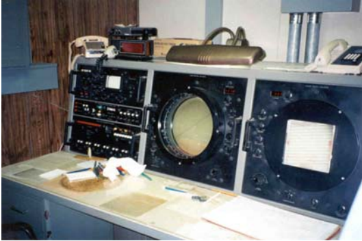
Figure 1 - WSR-74C 5 cm Radar in use at WSO Springfield IL prior to 1995. (Picture Courtesy NOAA/NWS North Webster IN.)
