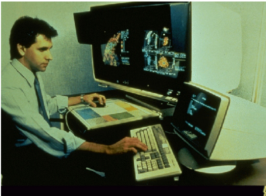
Figure 2 - WSR-88D Principal User Processor workstation in use at WFO Lincoln IL from 1995 to 2002. (Picture Courtesy NOAA/NWS Milwaukee WI.)
