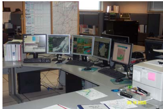
Figure 3 - Advanced Weather Interactive Processing System workstation used to integrate multiple meteorological datasets at WFO Lincoln IL since 1998.
