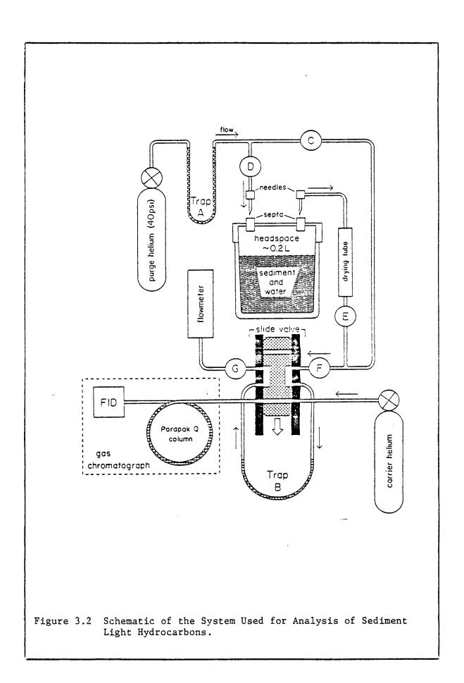
heated, injected into the carrier stream by a pneumatic slide value, and the hydrocarbons separated on a 3 m, 1.5-mm inside diameter (I.D.) Porapak Q column thermostated at 60°C. A flame ionization detector was used in conjunction with an electronic integrator for the analysis of sediment LMWH concentrations. A typical chromatogram showing separation of the gases is shown in Figure 3.3.
