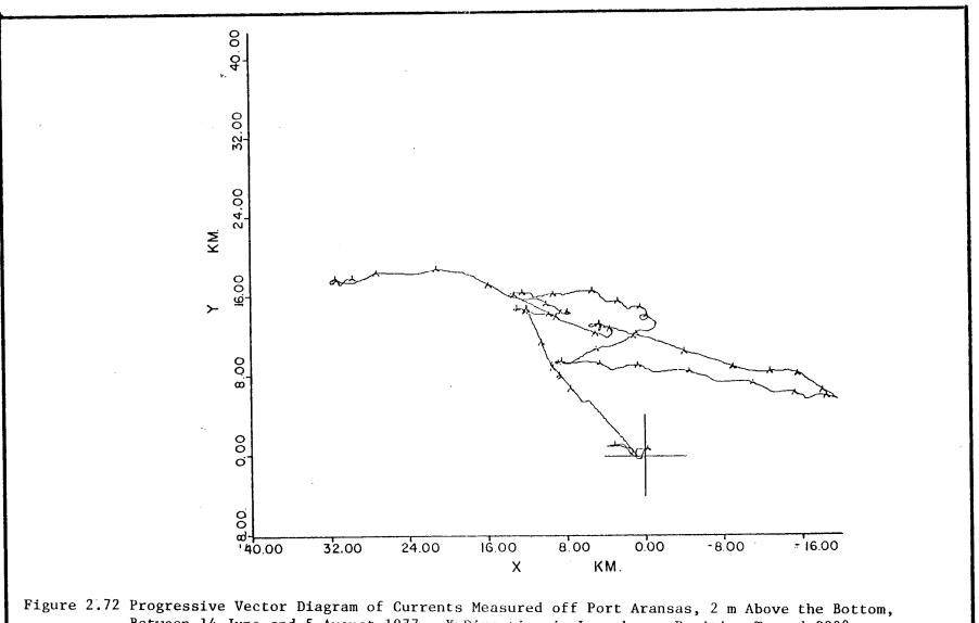
Between 14 June and 5 August 1977. X Direction is Longshore, Positive Toward O33°; Y Direction is Positive Offshore.
