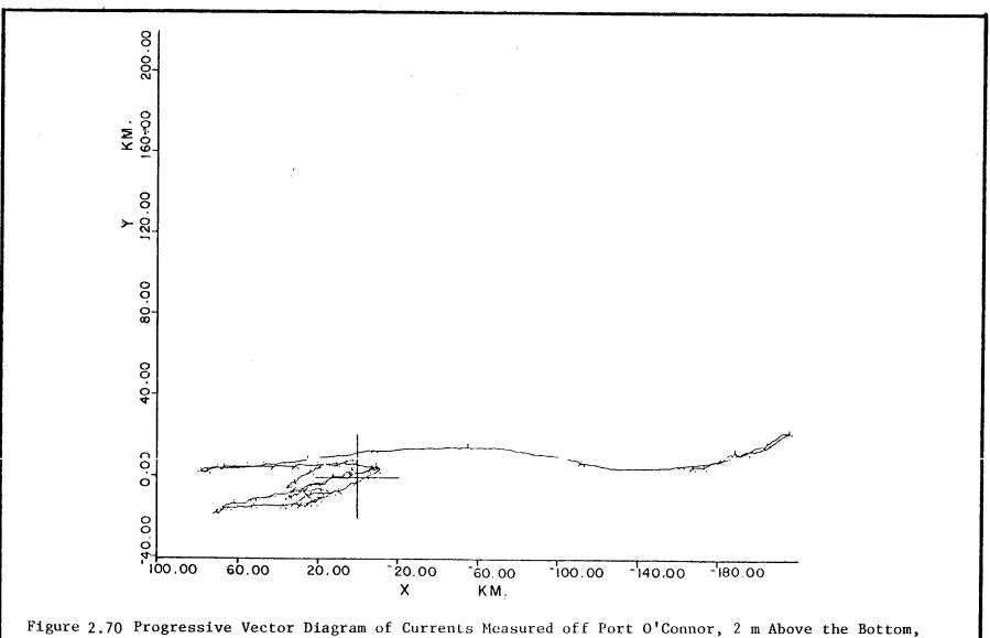
Figure 2.70 Progressive vector Diagram of Currents Measured off Port O'Connor, 2 m Above the Bottom, Between 22 June and 11 September 1977. X Direction is Longshore, Positive Toward 0.62°; Y Direction is Positive Offshore.
