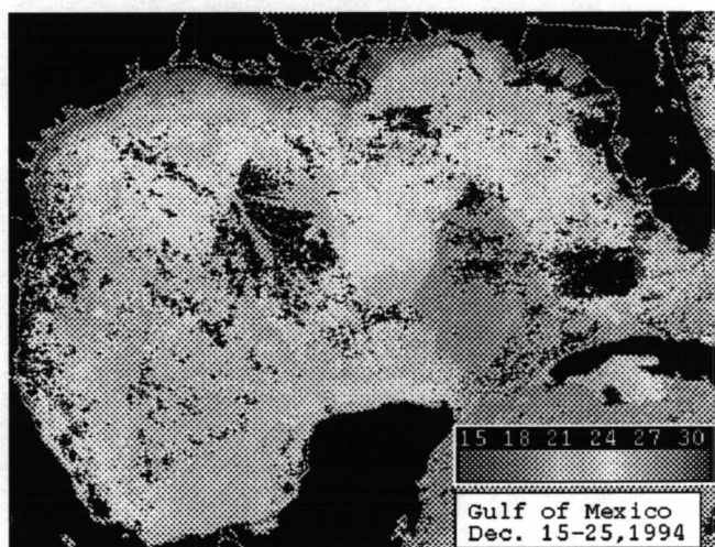
Figure 10 A composite of SST in the Gulf of Mexico derived from AVHRR imagery for December 15 to December 25, 1994
