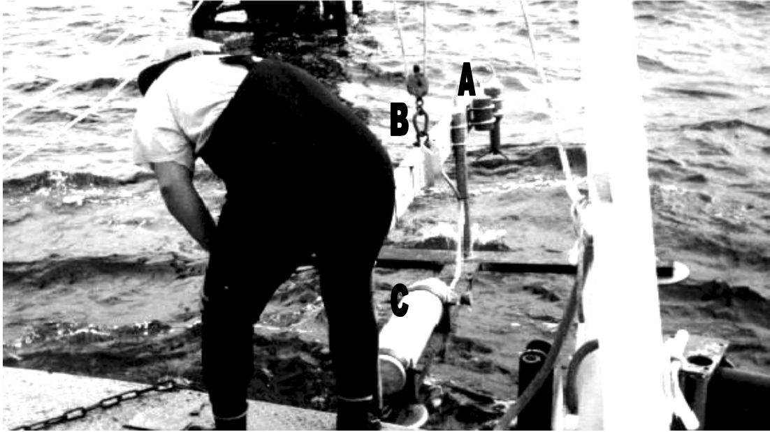
Figure 3.1. System 2A during deployment at Site 2. Key: (A) Acoustic Doppler Velocimeter (ADV); (B) Pressure Sensor; (C) Enclosed cylinder containing recorder module, compass and power supply. System 1A was identical except that it did not include a pressure sensor.
