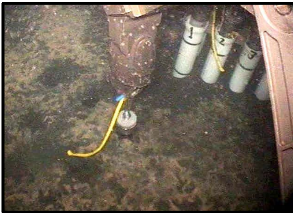
Photo 4. Sediment sampling with the ROV at a discretionary sample station with suspected Beggiatoa spp. on the surface.
