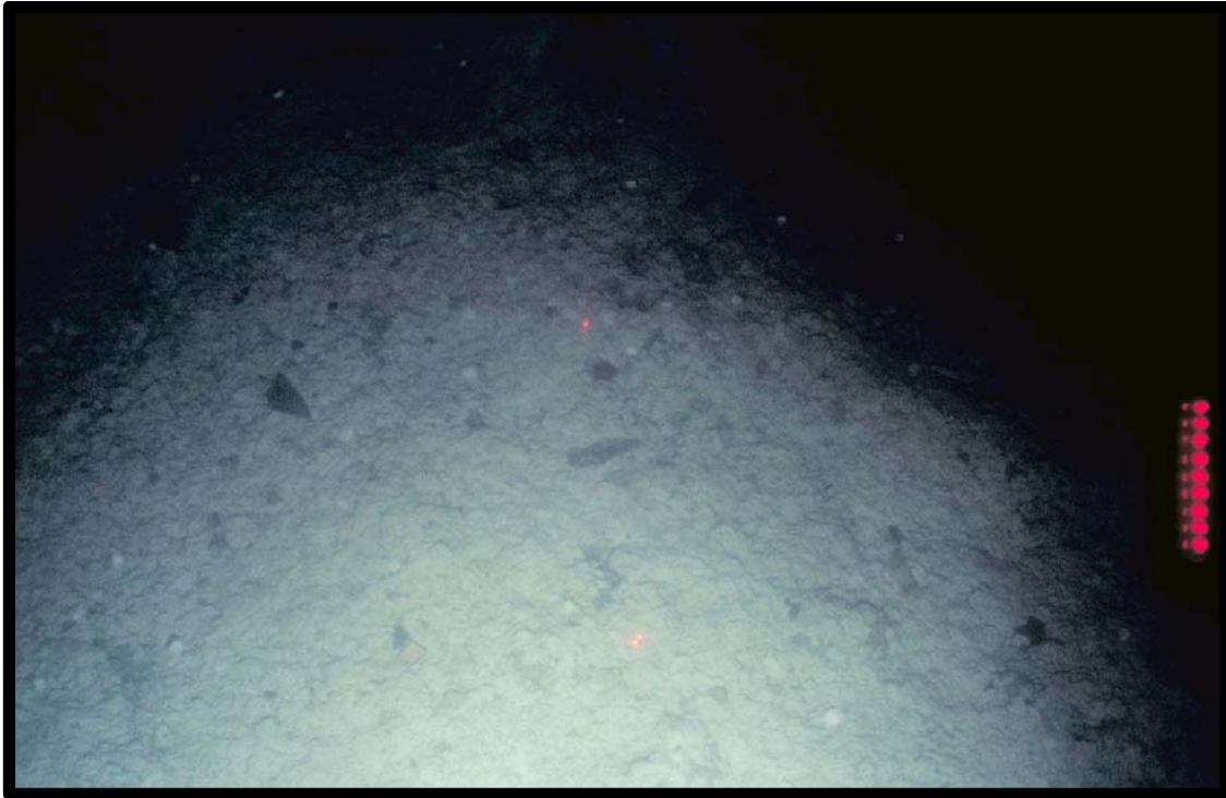
Photo 3 - Small mound along south side of Ewing Bank Area Block 305 platform. Sediment appears to be composed of muds and coarse cuttings.
