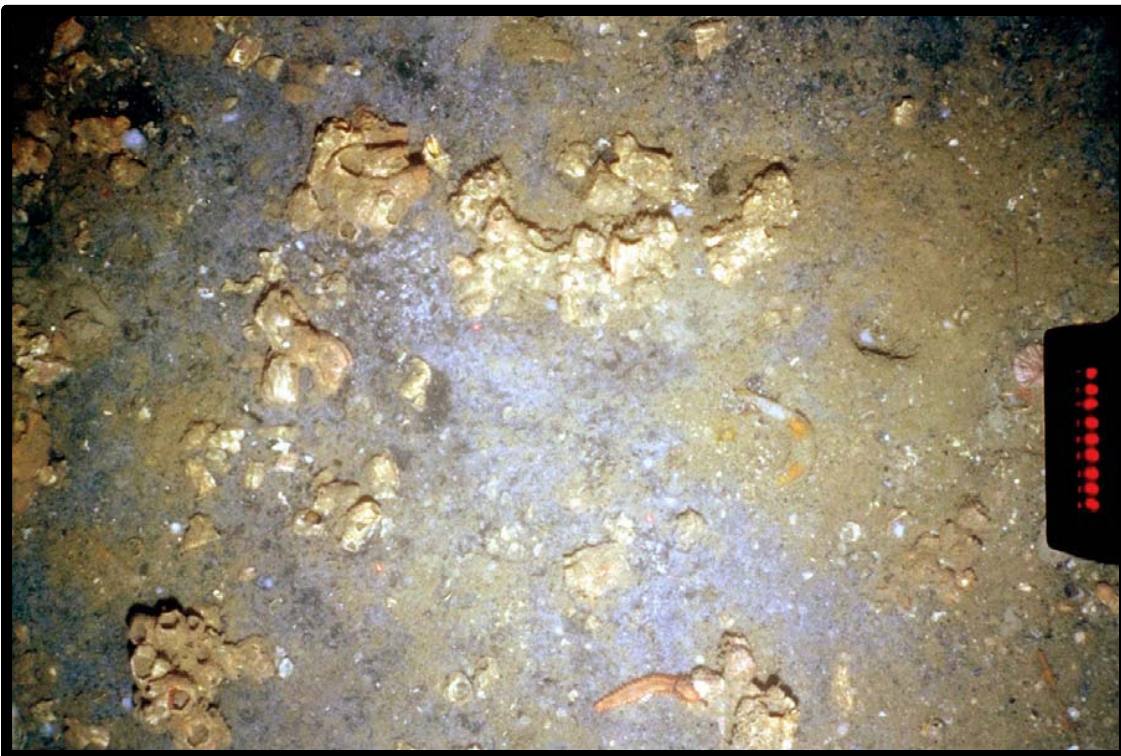
Photo 30 - Sediment in close proximity to the Main Pass Area Block 299 platform consisted of sand and mud with some coarse calcareous and ferrous debris.
