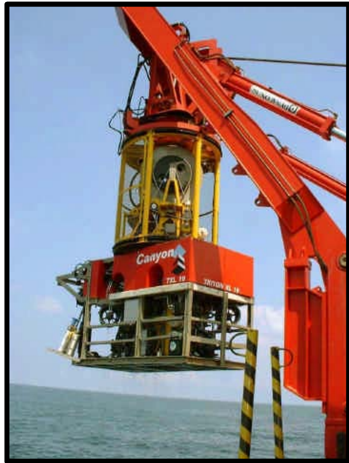
Photo 10. ROV and tether management system deployment.
