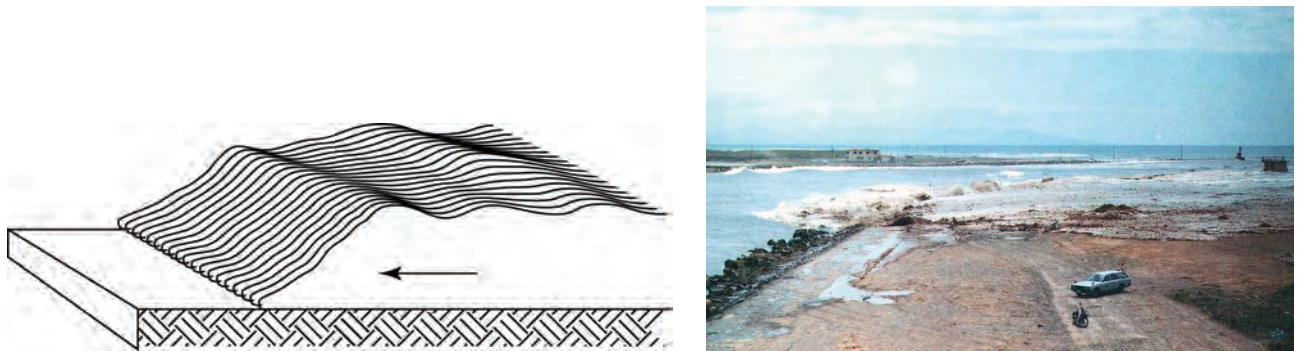
Figure 2-6 Sketch of a surge and photo of the 1983 Nihonkai-Chubu Tsunami showing the formation of a surge (Photo courtesy of N. Nara).
