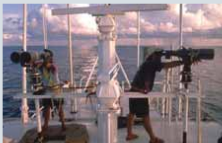
Binoculars known as “big eyes” are key instruments for marine mammal visual surveys.
