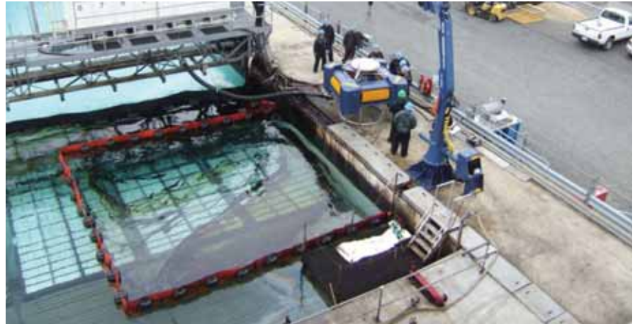
Above: The manifold and oil distribution system above the collection tanks on the bridge. The photo also shows one of the skimming heads being lifted out of the tank with the new crane system. Left: Skimmer heads being tested.
