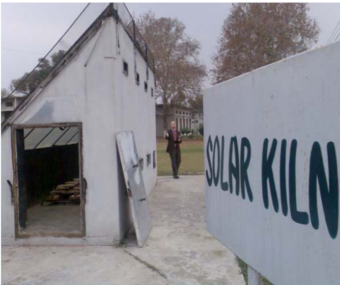
Solar Kilns are an inexpensive, accessible way of reducing the required time to dry wood from 2 years to a mere two weeks, while achieving uniform moisture levels
