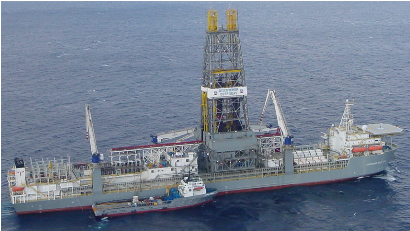
Figure 30. The Discoverer Deep Seas , a Class 1A1, double-hulled, dynamically positioned drillship (photo courtesy of Transocean).
