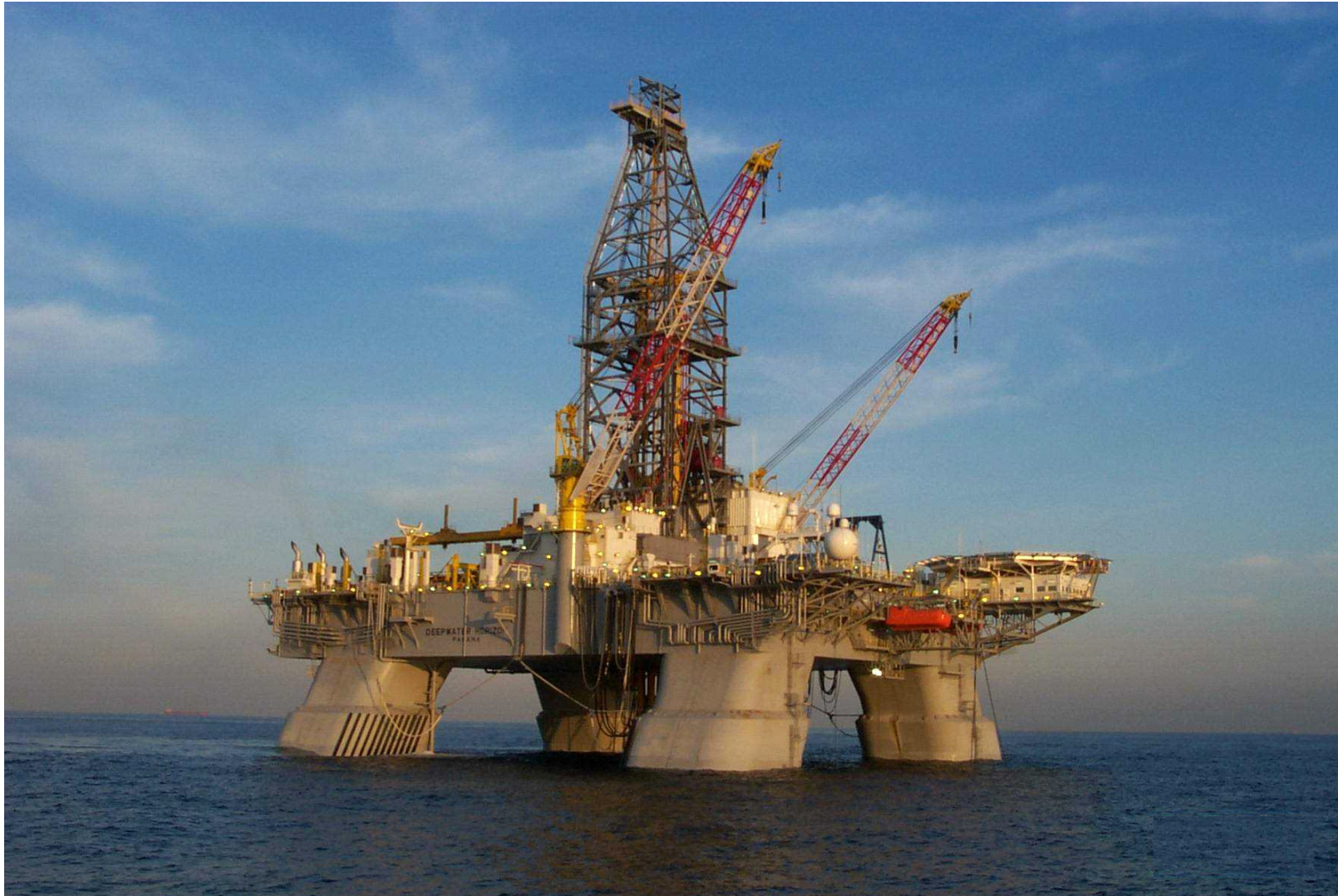
Figure 29. The Deepwater Horizon , a dynamically positioned, semisubmersible drilling unit (photo courtesy of Transocean).
