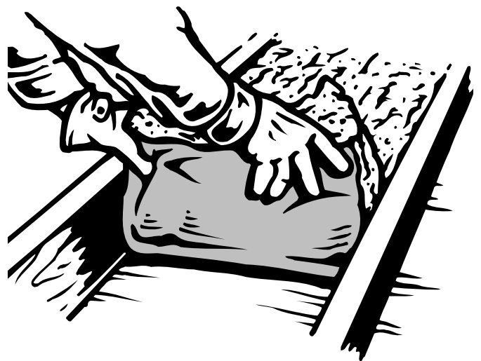
Figure 3. Correct installation of batt insulation
